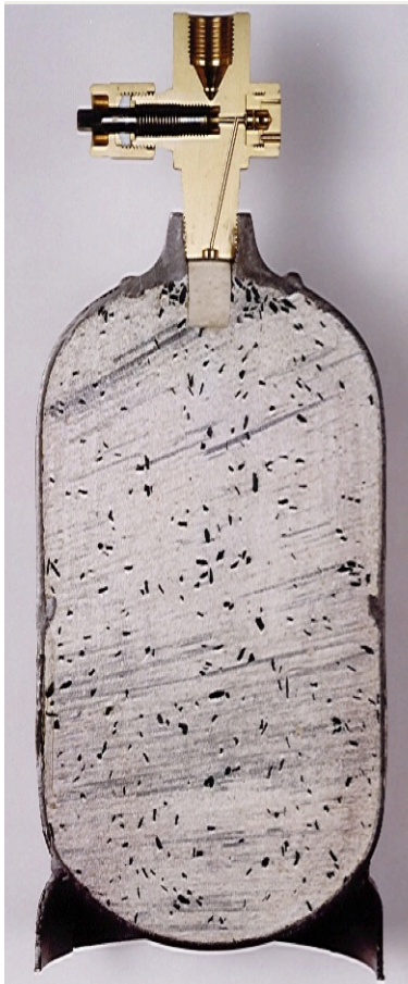
Figure 1: Cutaway photo of an acetylene cylinder
